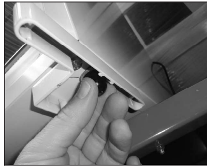
10. Gain access below bottom hinge, unscrew foot and...
