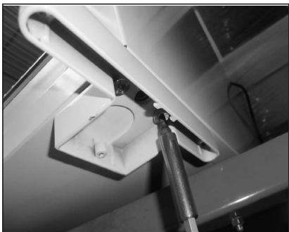
11. ...demount screws. Then remove bottom hinge and remount in new hinge side when ready
