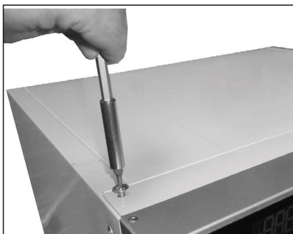
17. Remount four screws into toppanel
