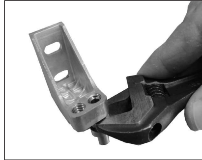
8. Unscrew the top hinge pivot with a spanner
