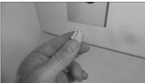
5. Re-seal both porthole ends with putty and remount service hatch (inside) + back-cover
