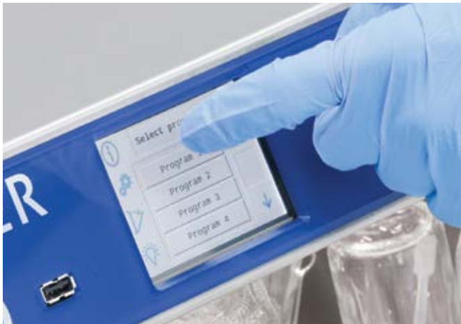
The Prolux PLC Controller includes a touchscreen interface with a common icon directory that permits scrolling access to primary screens from the same menu. A set of sub-menu screens display additional icon directories specific to the screen functions.
