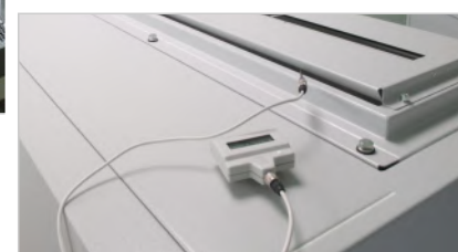
Temperature measurements of outward airflow
